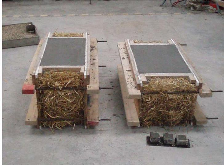
**Figure 5: Bales plastered on first side**
