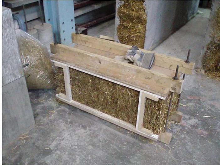
**Figure 3: Edging installed on a jig**
