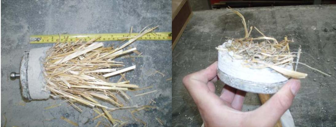
**Figure 9: Example of pull off disc from flat (left) and on-edge (right) wheat bales**
