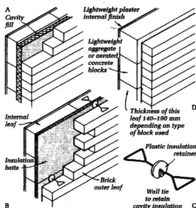
Figure 5.12 Thermal insulation of cavity walls
