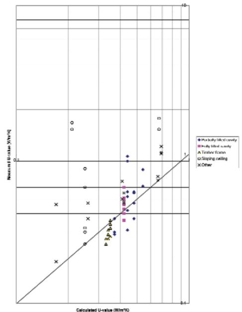
Figure 7: A graph of measured U-value against calculated U-value shown for various construction types. Those points which lie above the diagonal line correspond to the measured U-value exceeding the calculated U-value whereas the points which lie below the line are cases where the measured U-value is less than predicted
